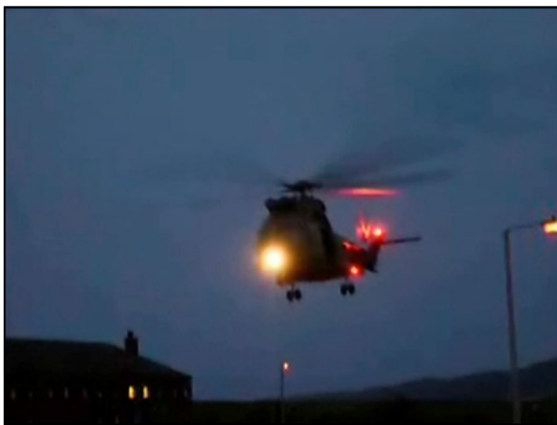
Figure 22: Landing lights of a SAE-330 Puma.
